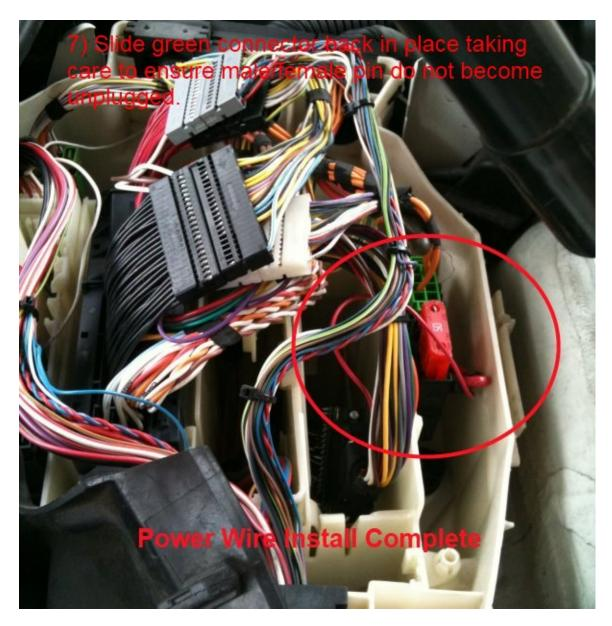
Ensure the male/female power wire connection is secure as you push the green connector down. If this connection comes loose while driving the motor will stall out and not restart.
