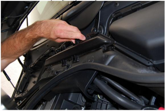
Release the left side tray by rotating the 4 plastic retaining bolts 1/4 turn.
