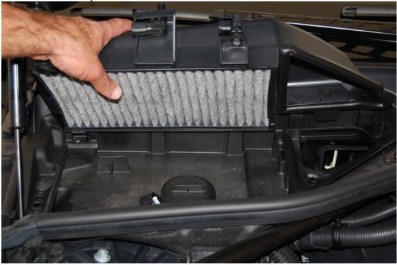
Pull off the weather stripping by pulling straight up and away until it has cleared the left tray, or about half way across the engine.
