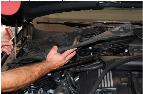
Use an allen wrench to remove the 5 screws holding down the ECU cover.
