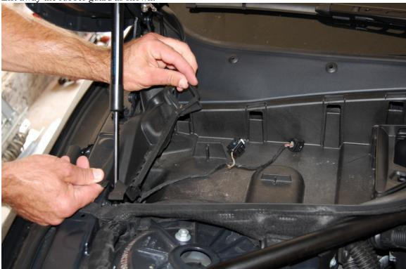
Remove the t25 torx screw holding the tray to the shock tower.
