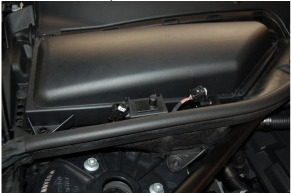
Use a 12mm socket unlock the plastic bolt by gently turning it 1/4 turn, and then release the metal latch holding it down.
