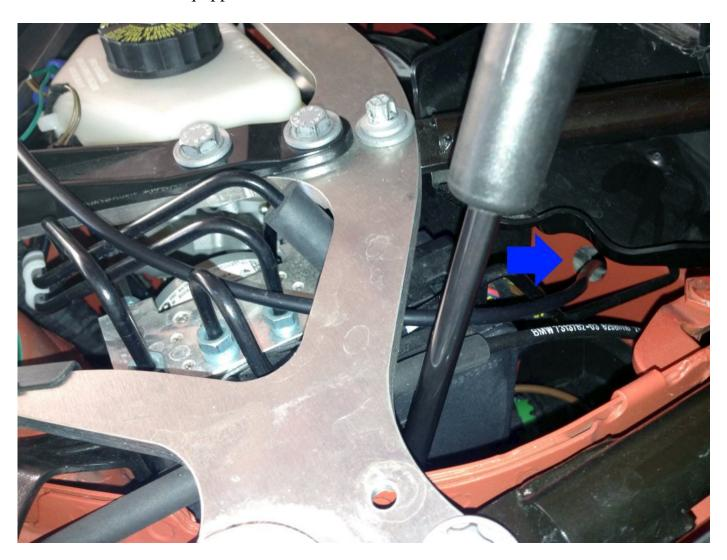
Plug the OBDII wire in to the JB4 green/brown molex connector.
