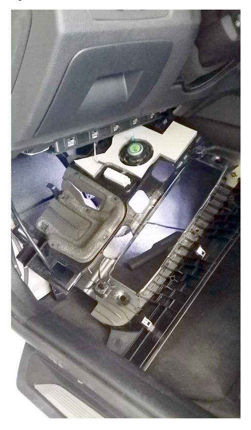
Using a long screwdriver push in on the rubber firewall cap pushing it in to the interior compartment. You'll see it fall down by the pedals and can put it away for safe keeping. Feed the OBDII wire from the interior through the hole to the engine compartment. Note this is also a great place to route your BMS DATA cable if equipped.
