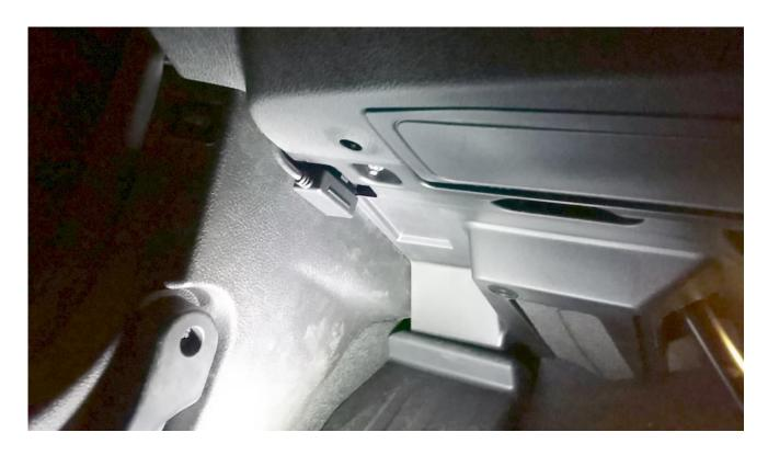
6) Tuck the now fully installed JB4 control box out of the way as shown. The wiring harness should be routed under the rubber cowl seal for a clean fit once the cowl cover is reinstalled. Tuck extra wire length out of the way taking some care to ensure nothing is too close to the moving mechanical parts of the windshield wiper arm/assembly.
