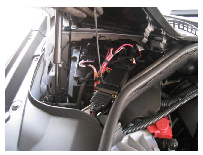
TMAP ground bypass required if USB cable touches battery rail, install wires with battery connected, etc. If you get a check engine light with the tuner completely removed you likely damaged the TMAP ground and need to perform this step to repair it. POSI-TAPS are on our website. While this is the quickest & easiest fix more detailed directions are posted to n54tech to repair the TMAP ground trace directly.
