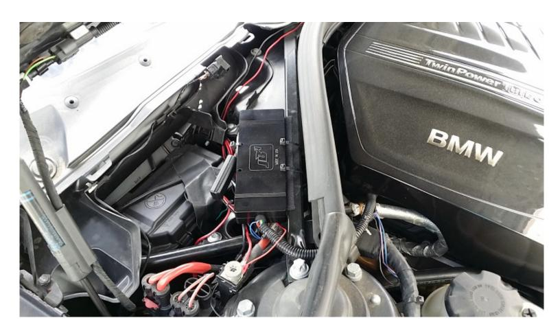
When reinstalling the cowl cover be sure it's fully seated and that you've lifted the rubber seal around it.
