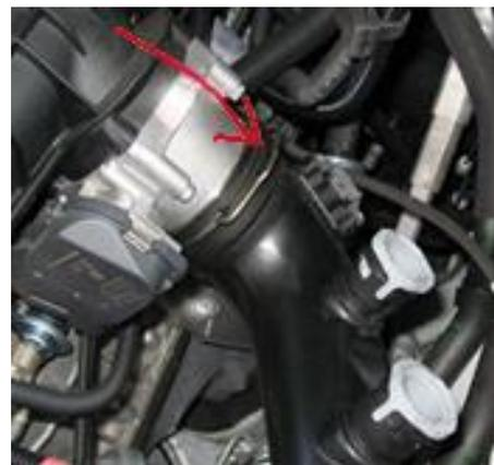
13) **Throttle Body** – There are 4 10mm bolts holding it to the intake manifold, remove them. On the bottom left-hand side you will find the wire harness plug – remove. Also, remove the vacuum line on the right-hand side in the same manner you removed the brake booster vac line.
