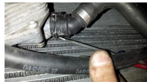
21) **Coolant** – From underside of engine you will see an aluminum box-like unit attached to the fan. Remove the locking clip from the small plastic fitting on the heater hose connected to it. Make sure you have a drain pan or a bucket with you to catch the coolant. Once drained, remove the T-25 Torx screw holding the aluminum box assembly from the fan. (sorry I do not know what this thing is called and it is driving me nuts)
