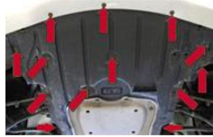
5) **Trans & Side/Corner Splash Shields** – need 8mm and 10mm sockets. These are the splash shields behind each wheel protecting the front strut rod bushings.
