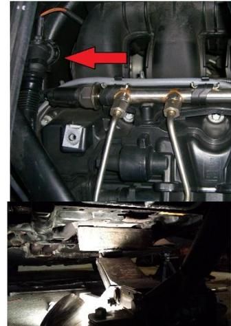
18) **FMIC Passenger-side clip** – using flathead remove this clip and disconnect hose from intercooler so it does not rip when lowering engine.
