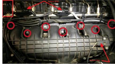
16) **PCV hose** – using a flathead screw driver and some patience, pry up each side of the plastic locking collar and wiggle off one side at a time.
