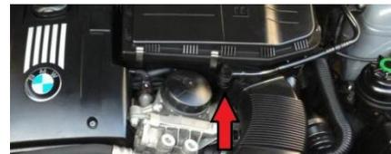
10) **Diverter Valves** – If you have OEM valves, turn the gray plastic lock collars to the left and lift up. Then pull vacuum line from intake manifold.
