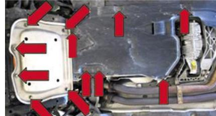
6) **Subframe Brace/Stiffener** – 6x 16mm bolts (aluminum pan in the picture to the right).
