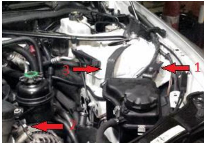
f. **Connect Coolant hose to bottom of overflow tank** – make sure to run this in away from the belt and pulleys.
