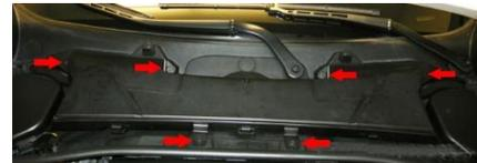
8) **Intake air filter snorkel** – remove 2 T25 torx screws from front of snorkel and pull up and out towards rear of car.
