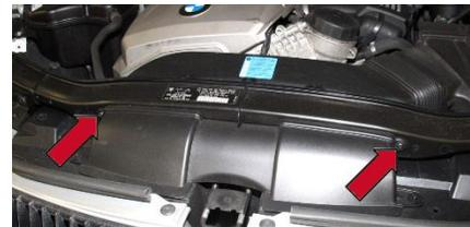
9) **Brake Booster Vacuum Line** – be careful, the clips on this are easy to break. Push in the sides and pull up gently. Then zip-tie to the side.
