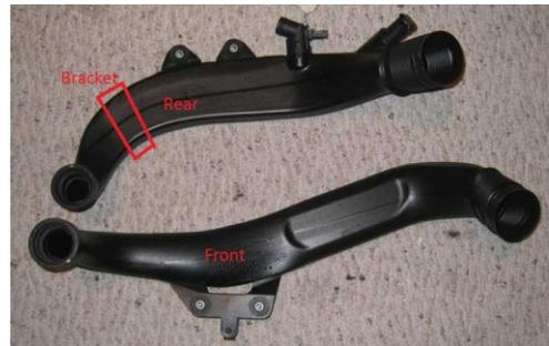
25) **Front Turbo Inlet** – there are two T30 torx bolts attaching the inlet to the front of the engine. Remove these and the inlet should slide right out.
