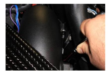
Passenger side intake is ready. Note strut bar is resting in position but not attached.
