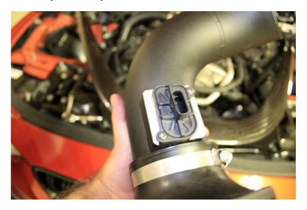
Install the Silicon piece first and tighten it down with the clamp provided.
