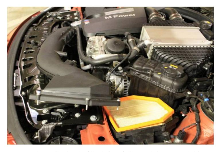
Remove your factory filter from the airbox but leave the OEM intake bottom tray. With the BMS performance intake its used as a heat shield and air duct.
