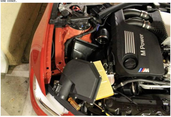
Remove the OEM accordion tube from the passenger side.
