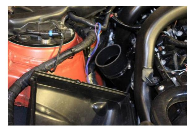
Install the filter on the BMS performance intake tubes.
