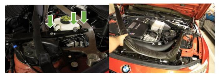
Remove OEM intake on the driver side. Remove clamp, Bracket, PCV, MAF sensor and the screws from the top portion of the intake system.
