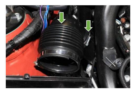
Transfer MAF sensors to the BMS intake using screws provided. Take care not to damage the MAF sensors as they are relatively delicate.
