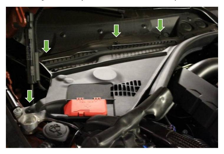
Remove the rest of the bolts from the struts bar and take it out put it aside.
