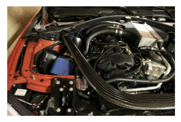
Install driver side intake. The filter rests on the OEM base.
