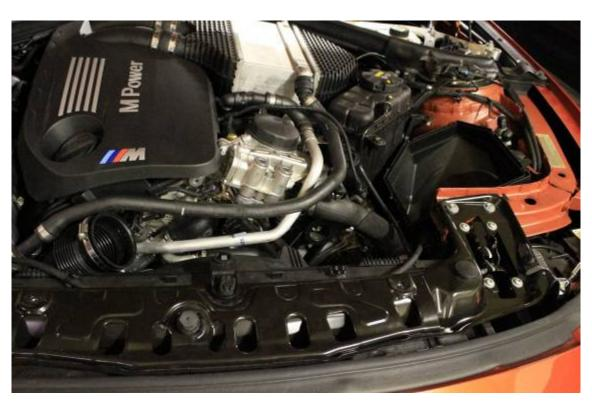
Repeat the same for the passenger side. Remove clap, MAF sensor and screws from the top of the filter.
