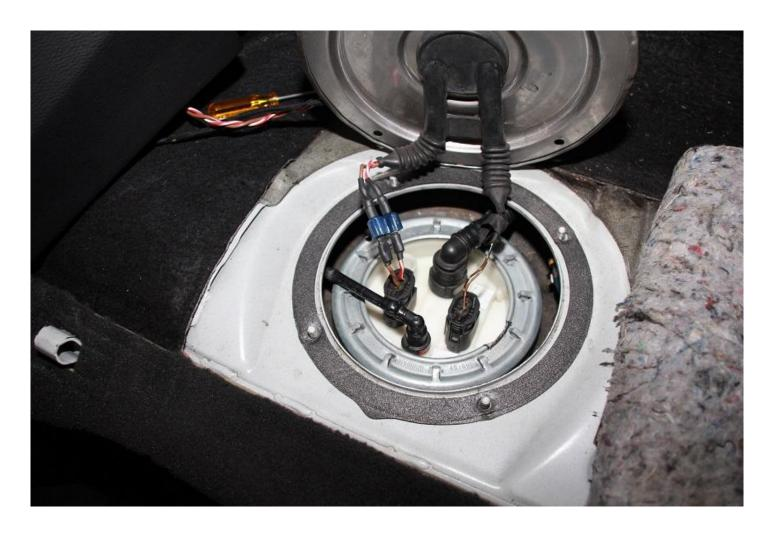
Install the access cover, replace the seat, reconnect the battery, and cycle power to the ignition a couple times to prime the fuel system.
