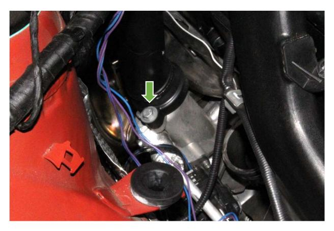
Unscrew the clamps connecting the intercooler and chargepipes.
