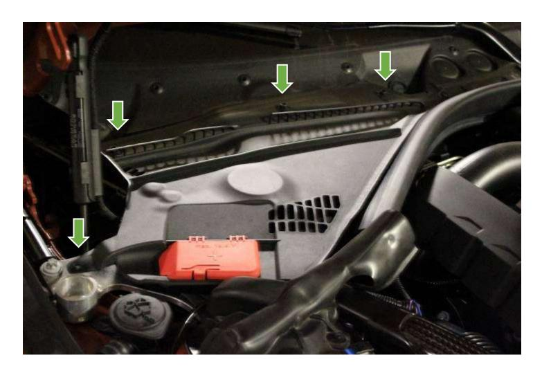
Remove the rest of the bolts from the struts bar and lift it out of the way
