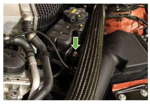
Remove the passenger/driver side cowl by removing the plastic rivet holding it to the aluminum brace and turning the three 10mm plastic bolts. Place the cover out of the way
