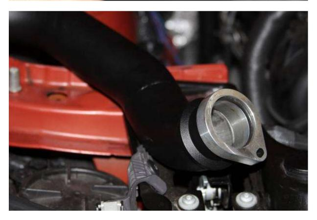
Install the silicon hose on the intercooler and tighten the clamp. Install the chargepipe to the intercooler then to the turbo outlet.
