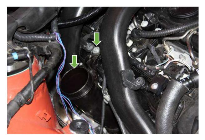
Now you can access the bolt to unscrew from turbo outlet.
