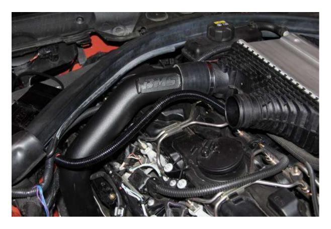
Tighten the chargepipe down with the screws provided with BMS chargepipe.
