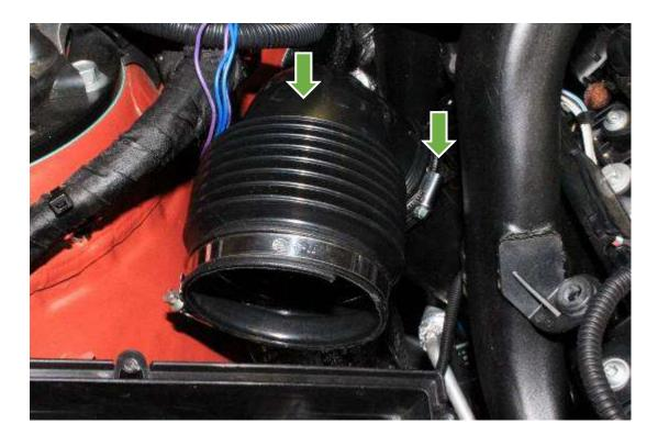
Unscrew bolt on the intake pipe and remove the plastic tube
