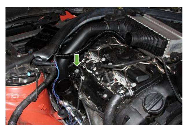
Install front chargepipe following the same steps as the rear pipe.
