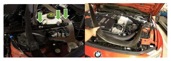
Remove passenger side airbox top and bottom.
