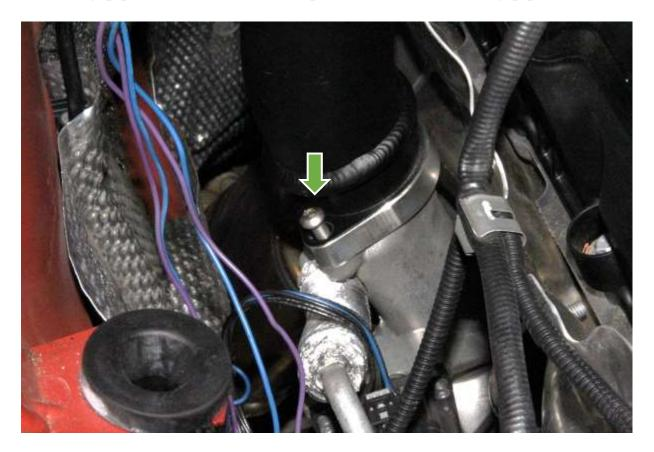
Tighten the clamp on the chargepipe.
