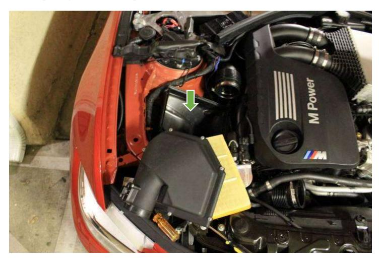
Remove the turbo inlet coupler
